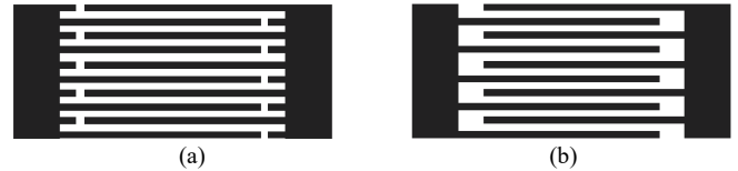
Fig. 6. Geometry of (a) IDT with dummy (b) IDT with wide gap
