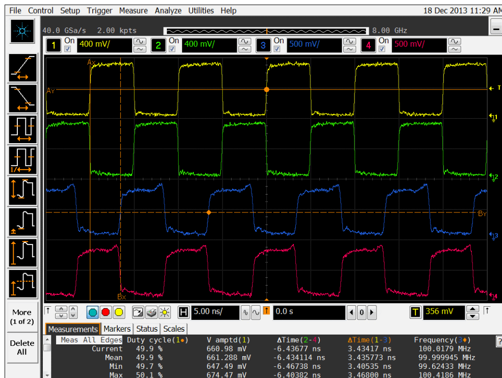
Figure 2. Input Clock vs. Output Clock of 1st Si53112, Bypass Mode
