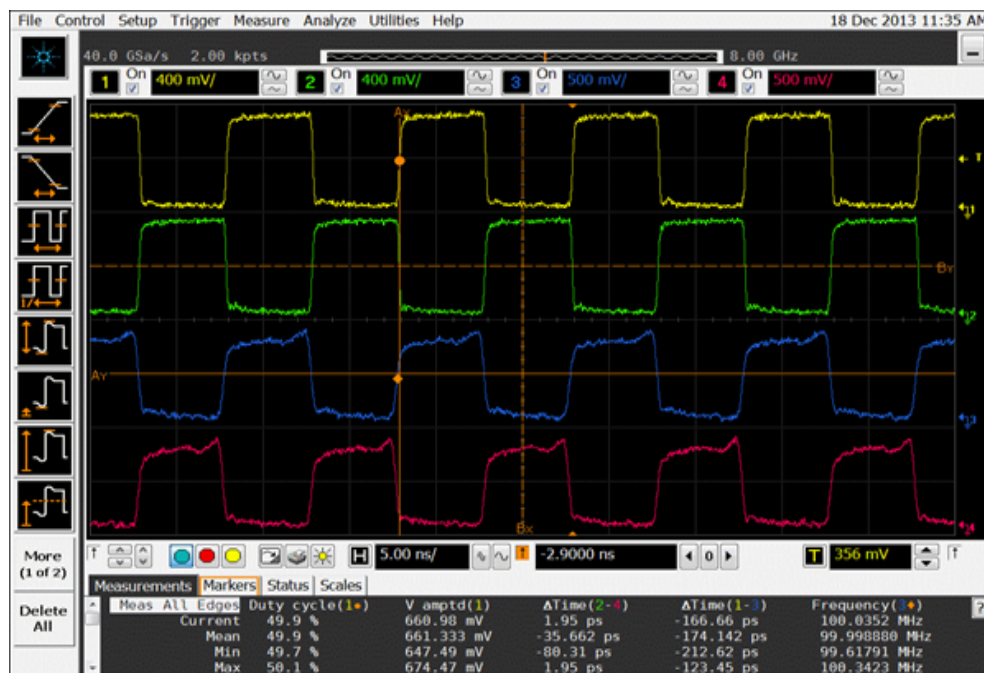
Figure 10. Input Clock vs. Output Clock of 2nd Si53112, LBW PLL Mode
