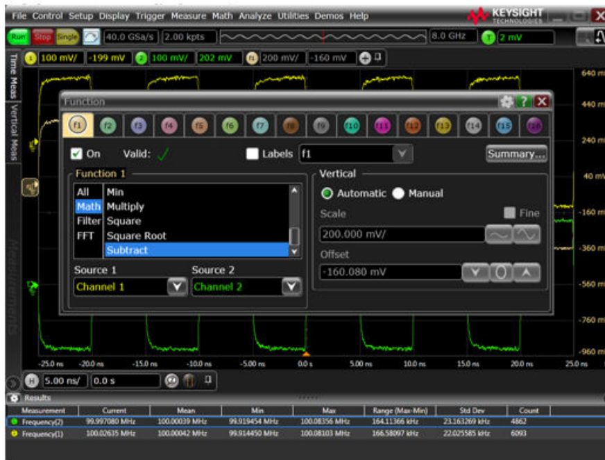
Figure 2.2. Creating a Differential Signal Using the Math Function (Part 2)
