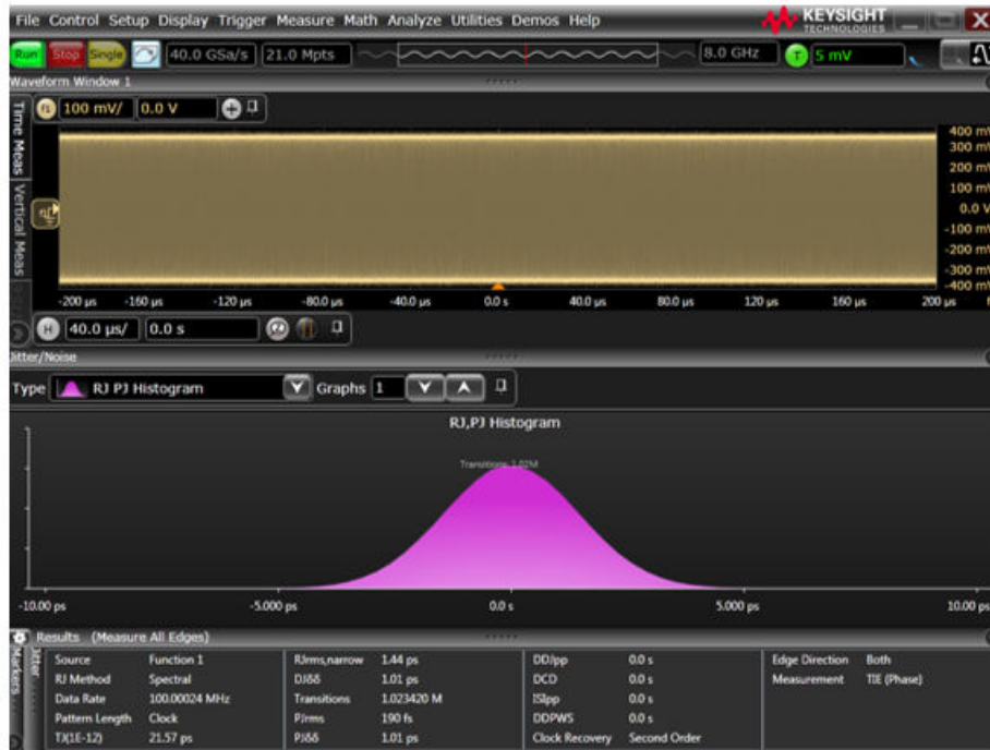
Figure 2.9. Capture Waveform Using PCIe Gen 3.0 Setup File
