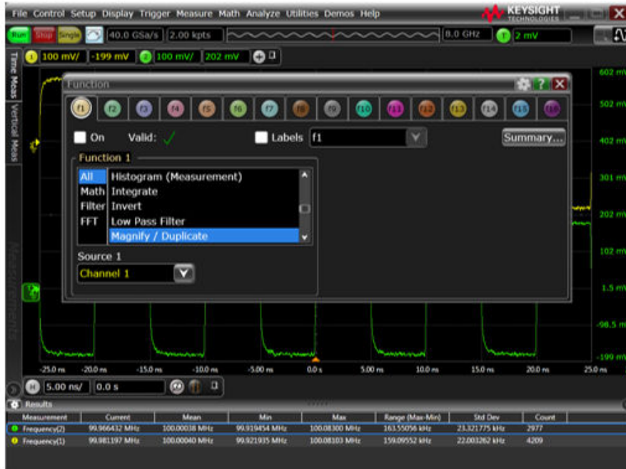
Figure 2.1. Creating a Differential Signal Using the Math Function (Part 1)
