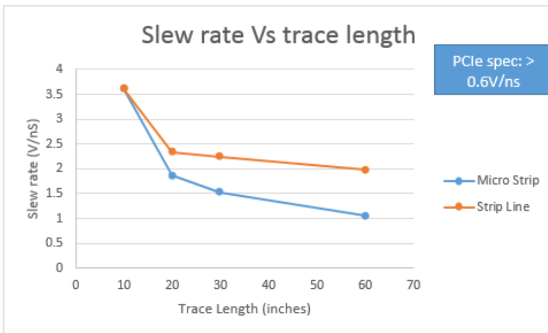
Figure 2.2. Slew Rate vs. Trace Length
