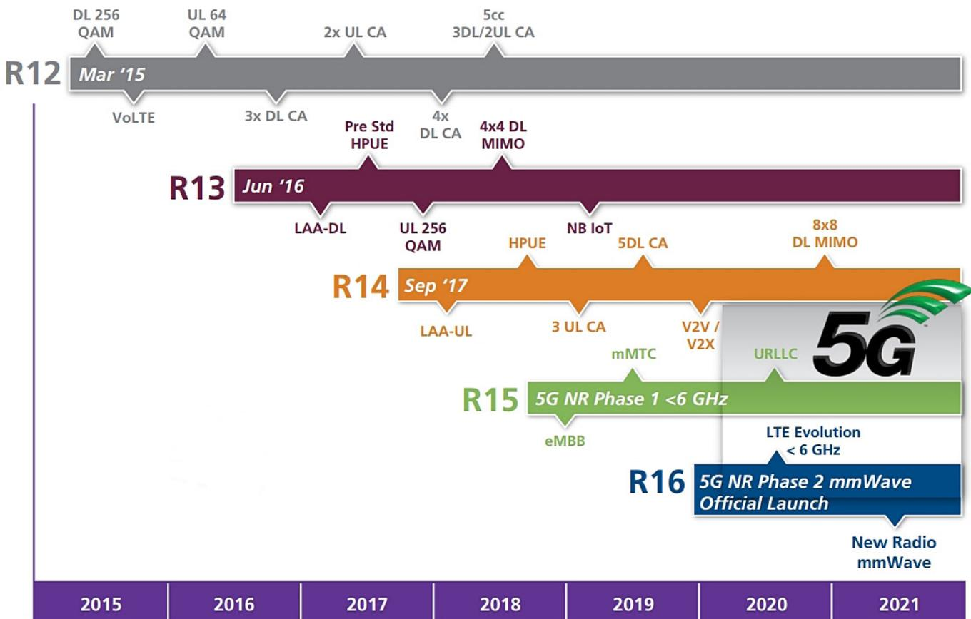
Figure 2. LTE and its evolution to (and through) 5G. Source: Skyworks Solutions
