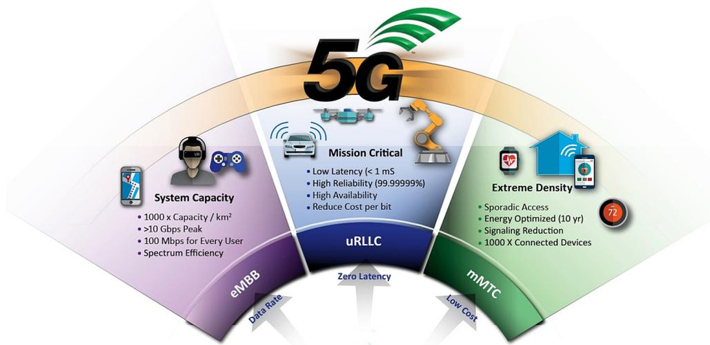
Figure 1. The three categories of 5G development: EMBB, MMTC, and URLLC. Source: Skyworks Solutions
