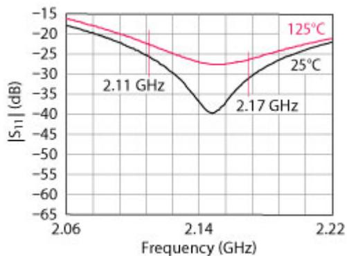
**Figure 3** Typical return loss of the isolator.
