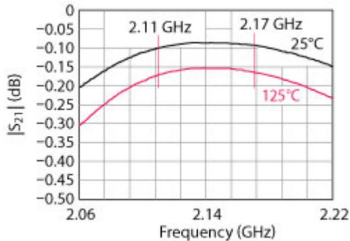
**Figure 1** Band 1 isolator insertion loss (SKYFR-001438).
