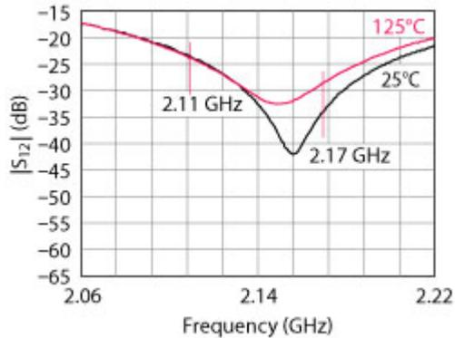
**Figure 2** Typical isolation of the isolator.
