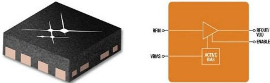
Figure 1. Skyworks' SKY67153-396LF LNA. Source: Skyworks Solutions
