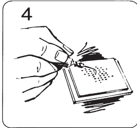
Remove chip from waffle at work station with vacuum pickup.
