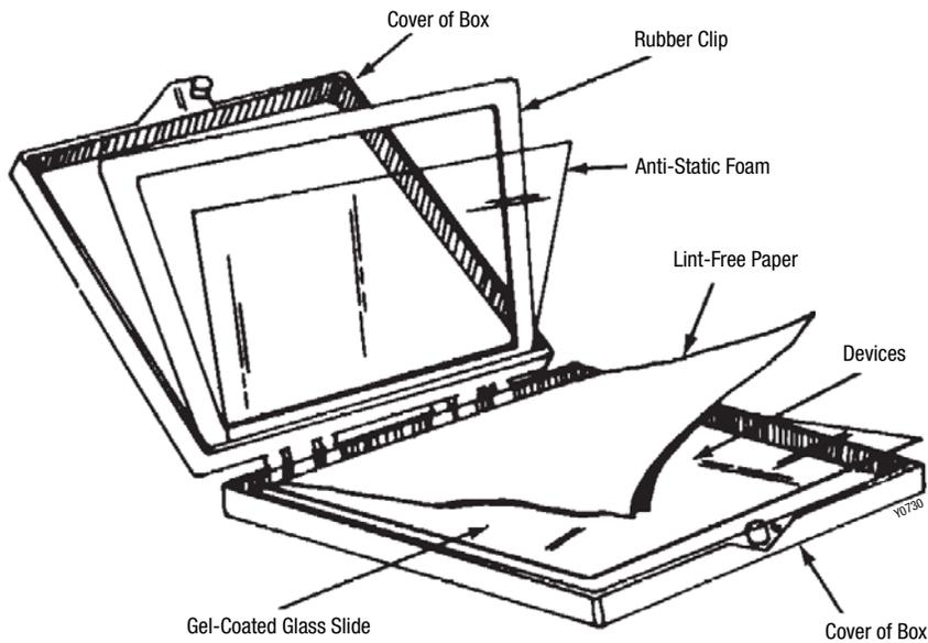
**Figure 5. Gel-Pak Beam-Lead Packaging**
