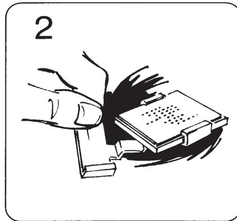
Remove both plastic fasteners.
