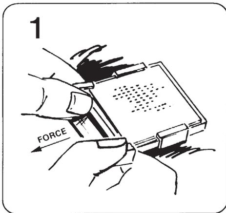
1. Place package on table top. There are two interlocking fasteners. Turn package so that interlocking side is facing down.
